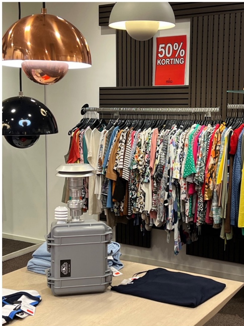
Air sampler and one Petri dish collecting microplastic in a clothing shop.
